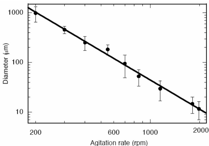
**Fig. 1. Average microcapsule diameter as a function of mixing speed.<sup>2</sup>**
