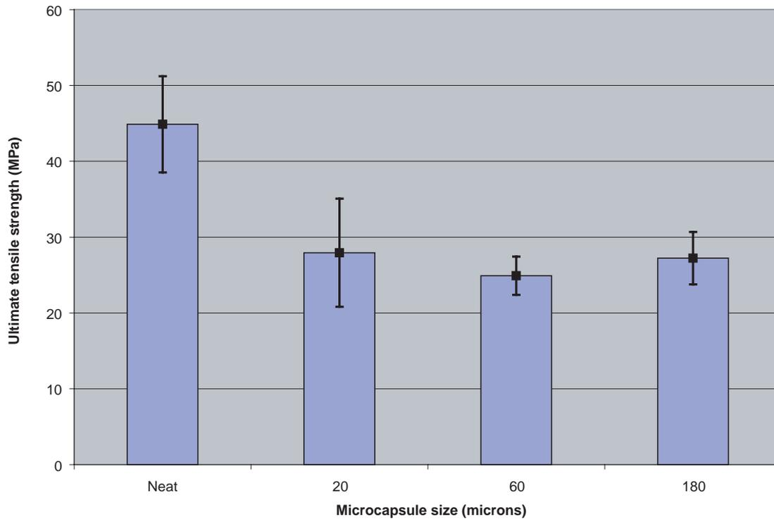
**Fig. 9. Ultimate tensile strength vs. microcapsule size.**
