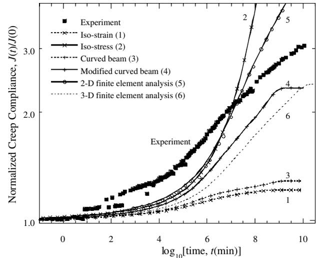
Fig. 5. Comparison of the experimental and predicted creep compliance along the warp direction for the micromechanical models.
