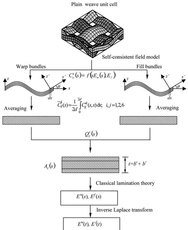
Fig. 3. Schematic of equivalent laminate model.
