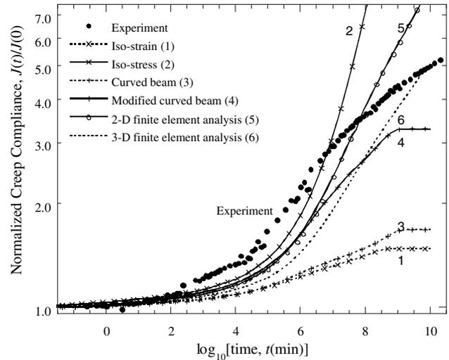
Fig. 4. Comparison of the experimental and predicted creep compliance along the fill direction for the micromechanical models.
