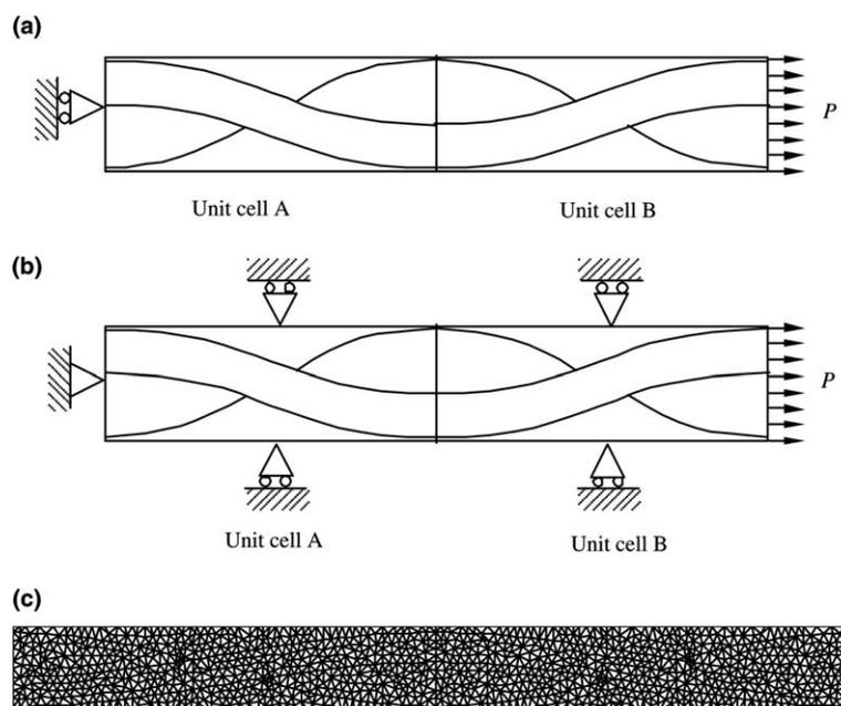
Fig. 7. Graphical representation of boundary conditions: (a) stress-free, (b) symmetric, (c) warp direction mesh of the two adjacent unit cells.
