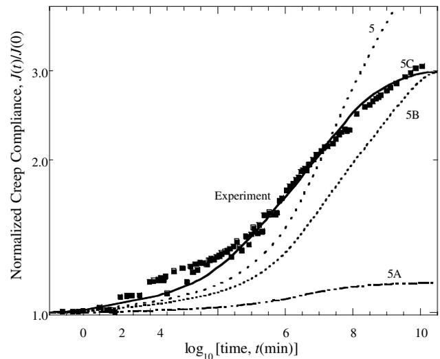
Fig. 10. Predicted creep compliance along warp direction for varying matrix response: (a) viscoelastic matrix with fixed Poisson's ratio, (b) elastic matrix in the fill and warp bundles, (c) viscoelastic matrix with constant bulk modulus and (d) viscoelastic matrix with constant bulk modulus and shifted retardation spectrum for matrix in fill and warp bundles.
