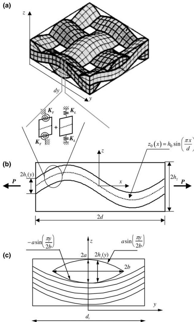
Fig. 6. Curved beam model: (a) schematic of the modulus calculation, (b) schematic of matrix load transfer, (c) Schematic of transverse crosssection.
