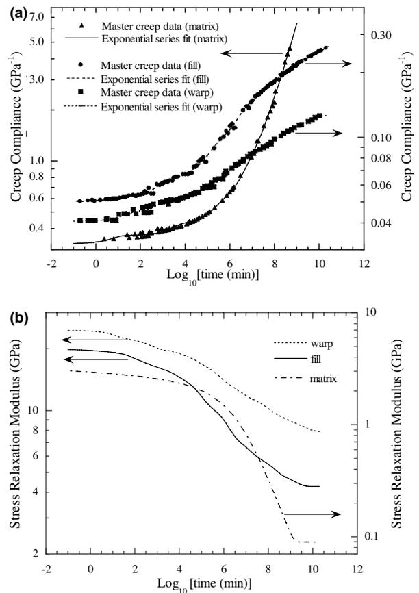
Fig. 2. Viscoelastic response of matrix and composite: (a) measured creep compliance of matrix and composite along the warp and the fill direction, (b) stress relaxation modulus of matrix and composite along the warp and the fill direction.
