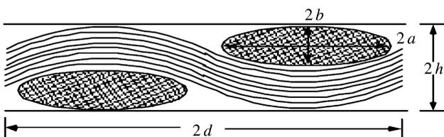
Fig. 1. Schematic of plain weave composite.
