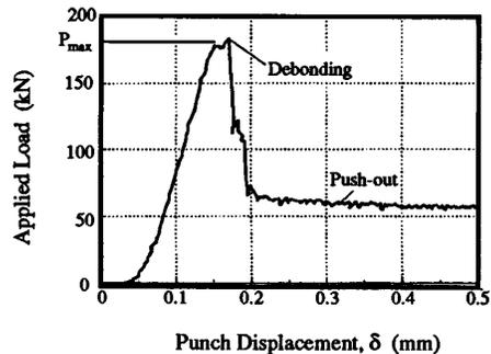
FIG. 4. A typical load-displacement curve for the push-out test.
