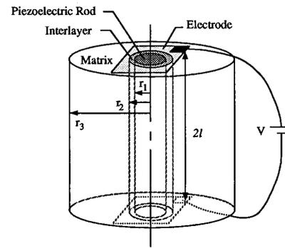
FIG. 2. Schematic of single rod sample for interferometric measurements.
