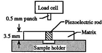
FIG. 3. Schematic of the thin section push-out test.
