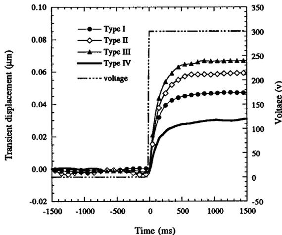
FIG. 5. Transient displacements measured at the center of the PZT rod.
