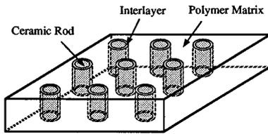
FIG. 1. Schematic of a 1-1-3 piezocomposite.
