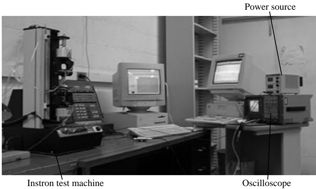
Fig. 2.5. Tension test setup.
