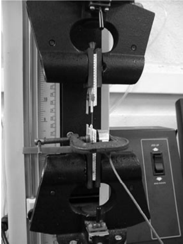
Fig. 2.7. AE sensor attached to specimen.
